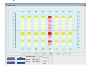
Visualisation of injection timing and injection duration for solenoid actuated injectors and valves.
