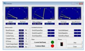
Overview on principle measured values and switch positions.
